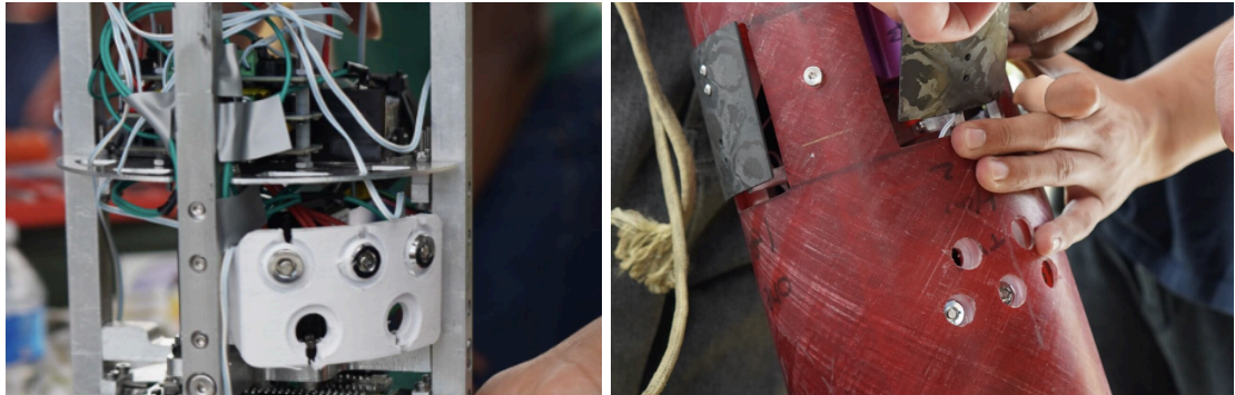
Figure 34. Avionics Bay with a Mechanical Key Switch Arming System
