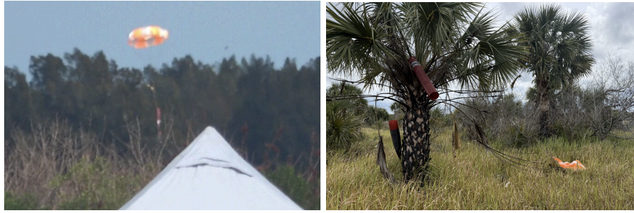
Figure 32. Recovery Sequence During Flight : (a) Main parachute deployment, (b) Post-flight landing configuration in field conditions.
