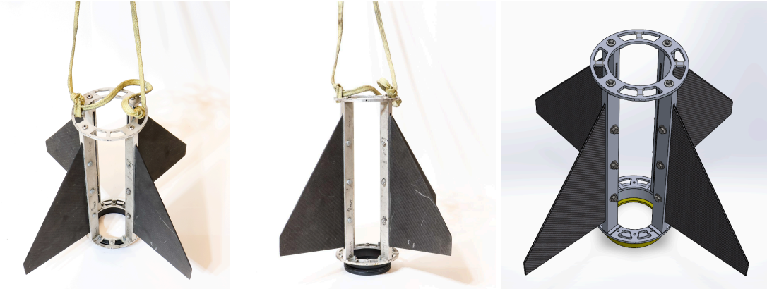
Figure 10. Modular Fin Assembly
