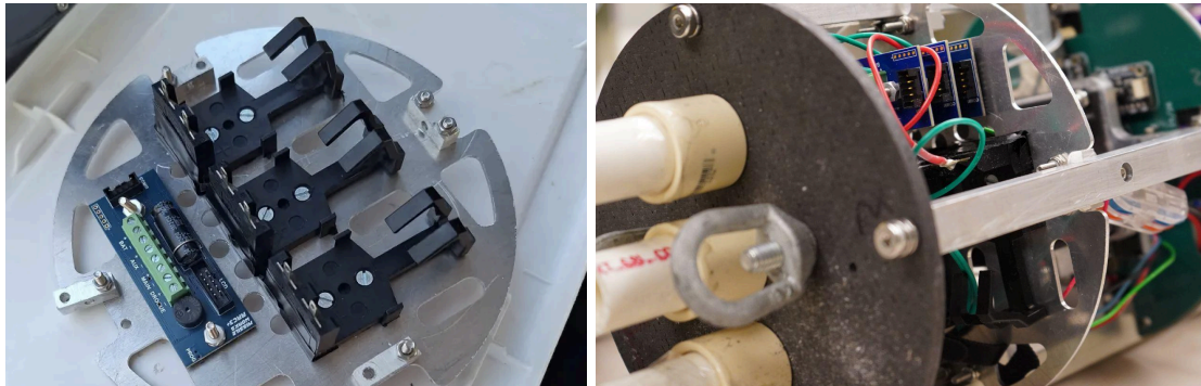
Figure 33. Triple-Redundant Recovery Avionics System: (a) Battery Mounting Plate showing three independent power supplies, (b) Integrated Avionics Bay with three RRC3+ altimeters
